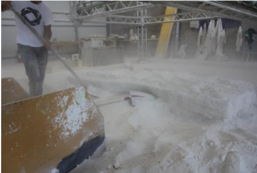
Removing of the powder bed from the printed object
