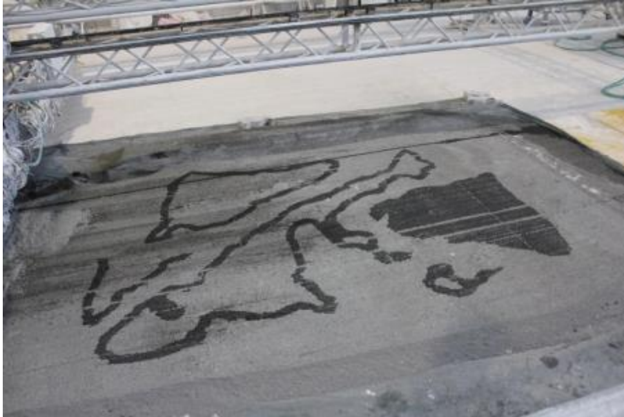
A layer being printed (dark gray areas indicate the deposited binder)
