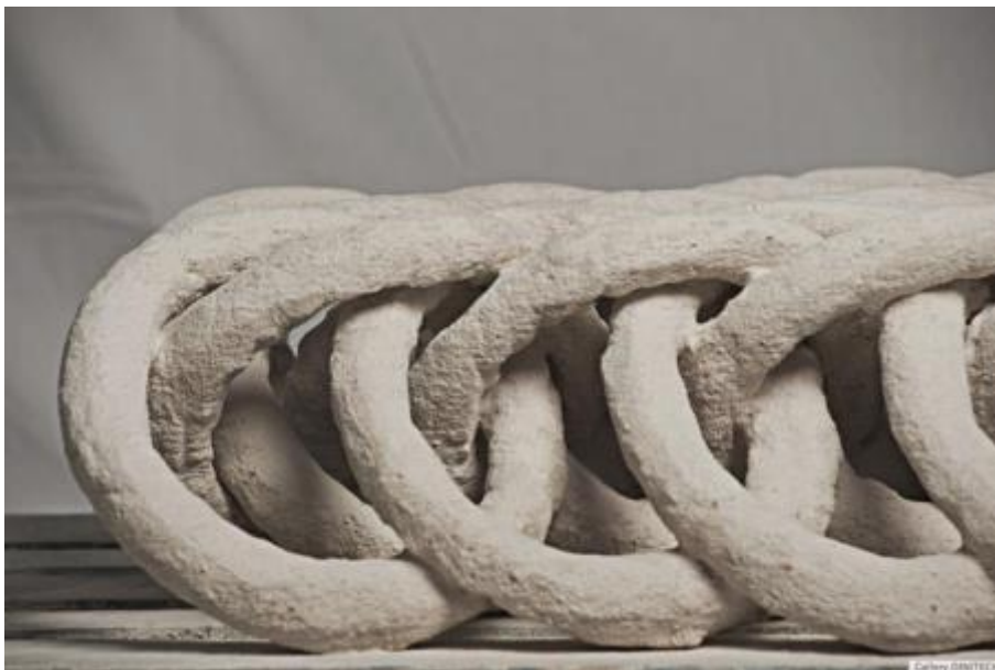
An intricate shape with linked rings, made possible because of the use of binder jetting technology
