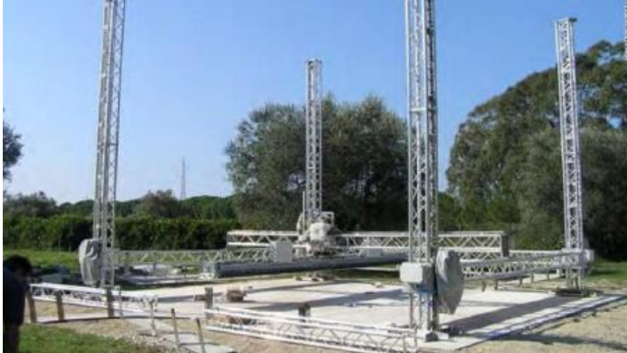
The D-Shape printer in outdoor conditions
