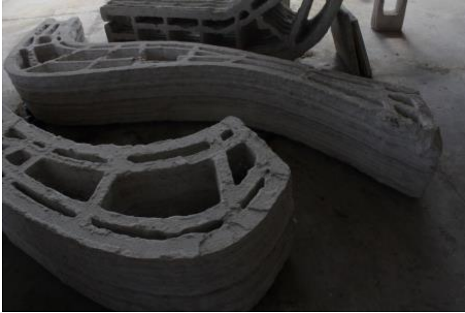
Components or test prints for Villa Rocca, a large organic villa project, to be used as stay-in-place formwork
