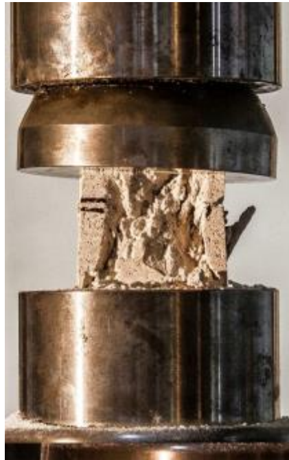
A specimen tested under compression load
