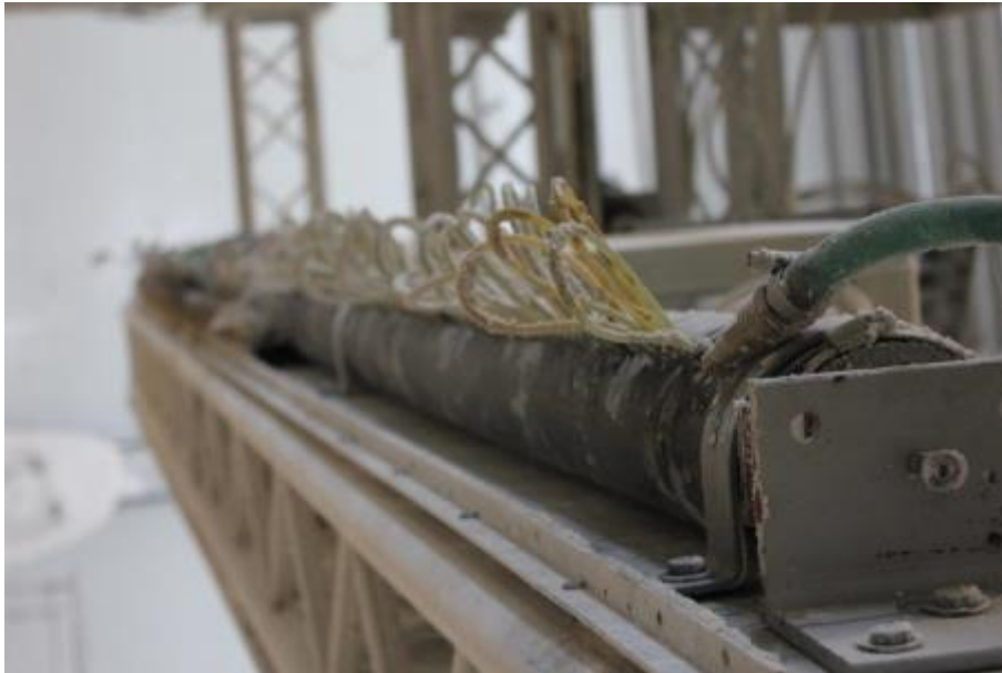
Feeding tank for the liquid component (with the feeding hose on the right)
