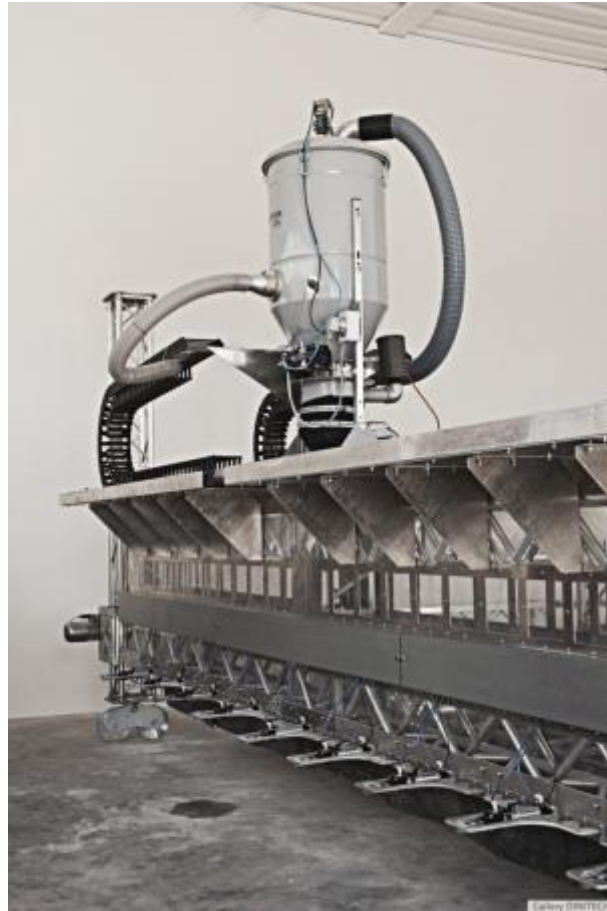
Sand feeder mounted on top of the printer gantry (2nd generation printer)
