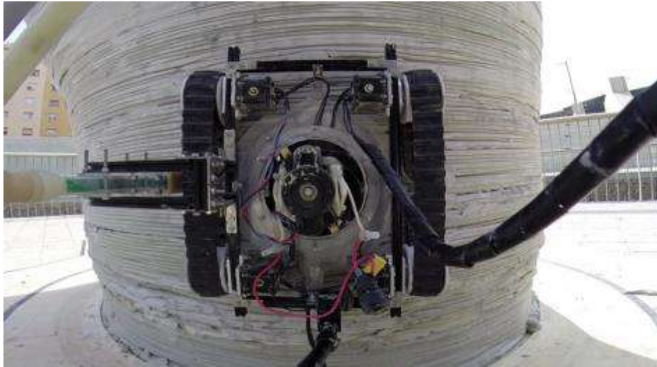
The Vacuum robot attached onto the vertical face of a printed object
