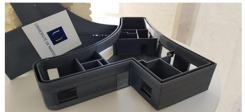
3D printed model of the house showing the plan layout and internal wall partitions.
