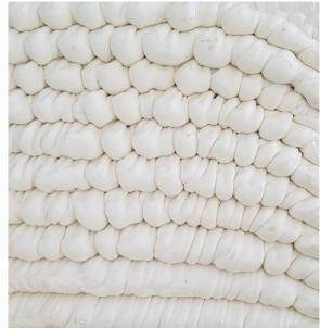
Approx a meter height of a portion of a wall sample printed in polyurethane.
