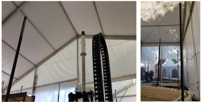
Laser beacon on top of the robot (left image) and laser receptors (right image).
