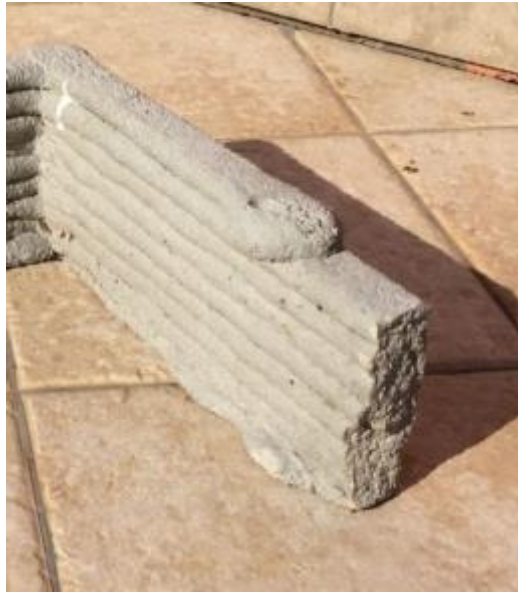
A cross section of the material showing a good bond between layers
