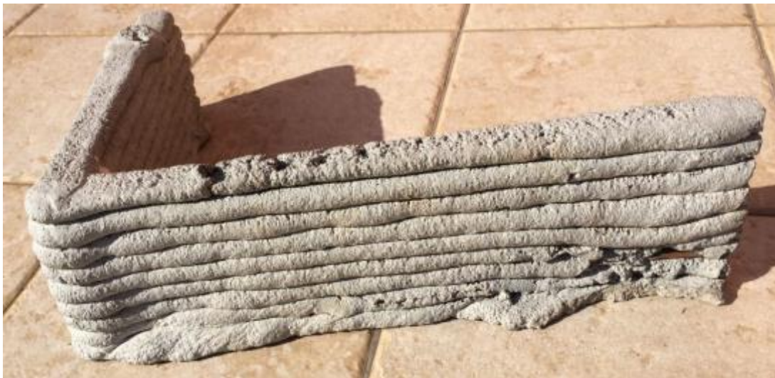
A sample of printed material with the distinctive layered surface, along with some errors and porous areas
