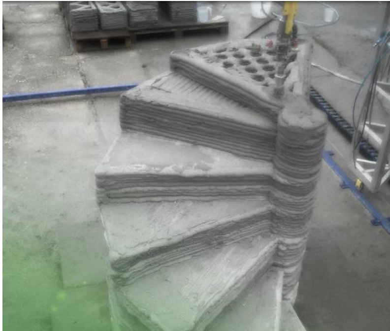
The staircase printed by BetAbram is an example of an object with 2.5D freedom
