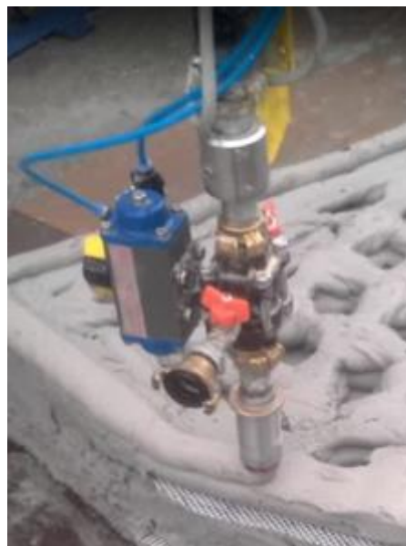
View of the two versions of the nozzle, one with a visible controller (left)
