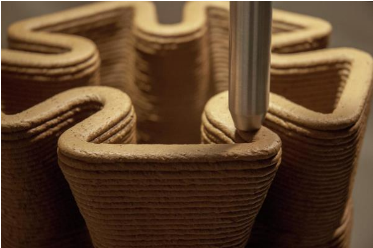
The Pylos 3D Printer extruding wet soil
