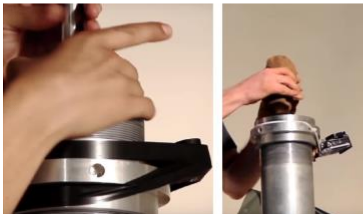
The procedure for feeding the material: nozzle unscrewing (left) and material filling (right)
