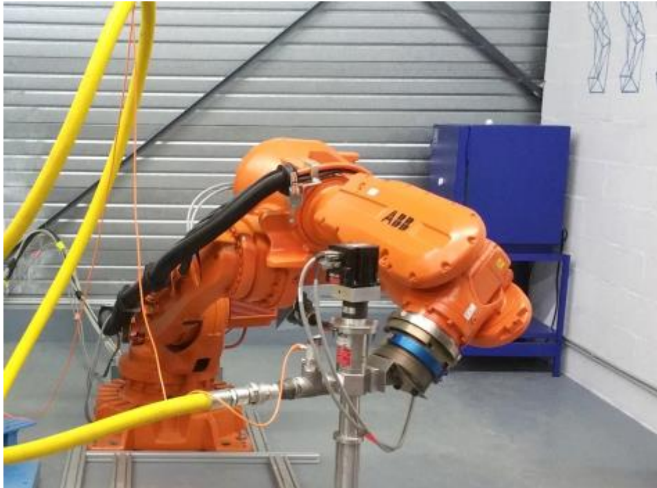
The Pylos deposition with piston on top, cylindric container in the middle, and nozzle in the bottom
