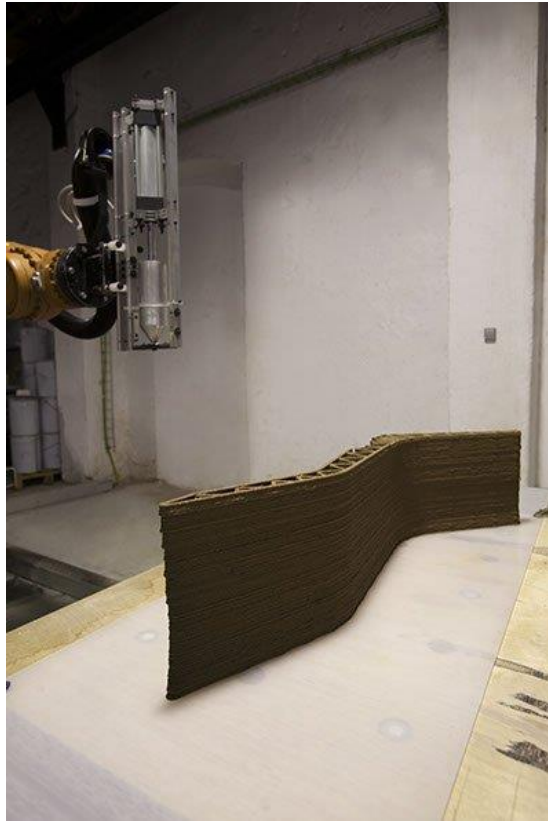
The largest prints of the Pylos project, an organic pile (left) and a curved surface segment (right)
