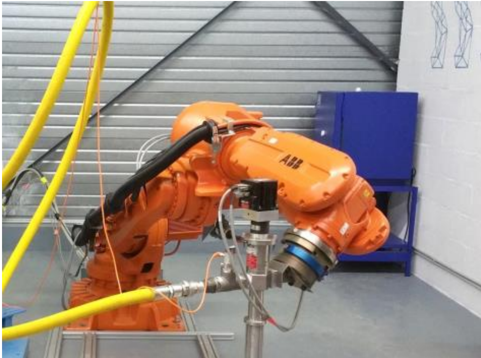
The material deposition system of an XtreeE printer
