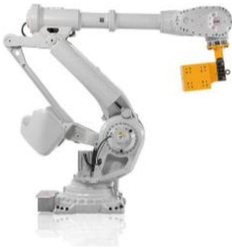
An IRB8700 robot from AAB (left), along with a sketch of the the six-axis of rotation (right)
