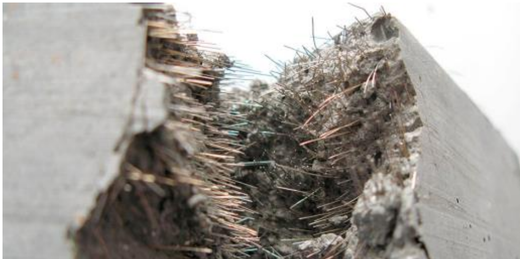
Ultra-high performance concrete (UHPC), with visible steel fibers.
