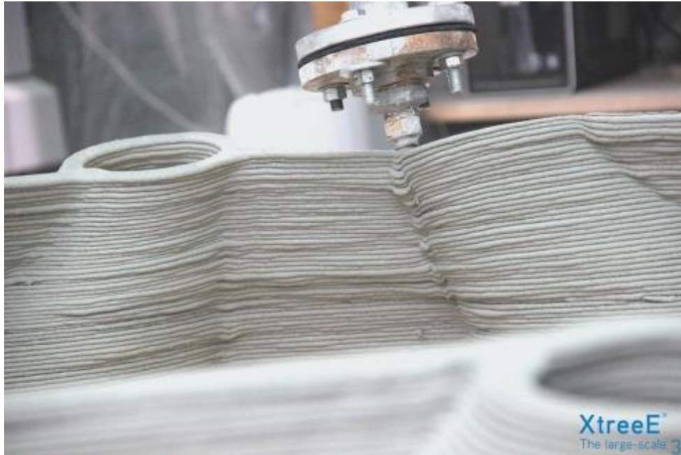
The XtreeE printer - printing of a layer
